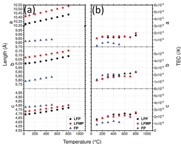
Fig. 7 (a) Lattice parameters of LFP, LFMP and FP in argon atmosphere depending on the temperature and (b) thermal expansion coefficient (TEC) as a function of temperature and the crystallographic axis of LFP, LFMP and FP.
