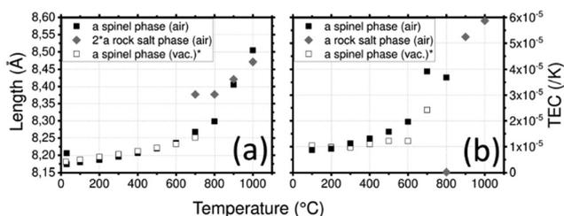
Fig. 6 (a) Lattice parameters of LNMO depending on the temperature and (b) thermal expansion coefficient (TEC) as a function of temperature and the crystallographic axis of LNMO. (\*) Calculated from data of Zeng *et al.*<sup>76</sup>
