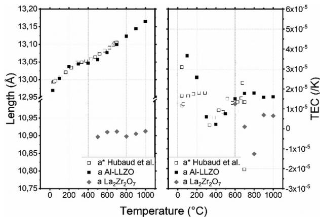
Fig. 4 (a) Lattice parameters of AL-LLZO and La<sub>2</sub>Zr<sub>2</sub>O<sub>7</sub> depending on the temperature in air and (b) thermal expansion coefficient (TEC) as a function of temperature and the crystallographic axis of AL-LLZO. (\*) Data from Hubaud *et al.*<sup>19</sup>
