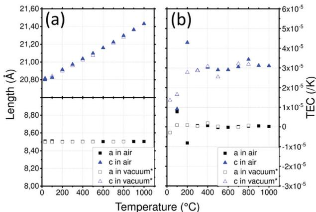
Fig. 3 (a) Lattice parameters of LAMP depending on the temperature and (b) thermal expansion coefficient (TEC) as a function of temperature and the crystallographic axis of LAMP. (\*) Data from Monchak *et al.*<sup>51</sup>
