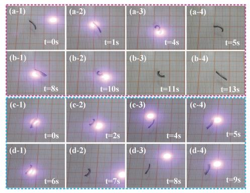
Fig. 6 The  $90^{\circ}$  circulatory and the homodromous circulatory switching processes of NFC2 gradient intelligent hydrogels. (a-1)–(a-4) Switching  $90^{\circ}$  to left and (b-1)-(b-4) switching 90° to right with a power density of 6.32 W cm<sup>-2</sup>. (c-1)-(c-4) The first, and (d-1)-(d-4) the second switching process with a power density of 18.7 W cm<sup>-2</sup>.
