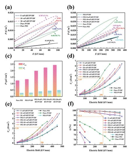
Fig. 5 P-E loops of (a) single layer composites and (b) bilayer composites with different BaTiO<sub>3</sub> loadings. (c) The maximum displacement  $P_{\text{max}}$ and remnant displacement  $P_r$  of the pure PEI and bilayer composites at 350 kV mm<sup>-1</sup>. (d) The storage energy densities, (e) discharge energy densities and (f) discharge efficiencies of the single layer and bilayer composites under varied external electric fields.
