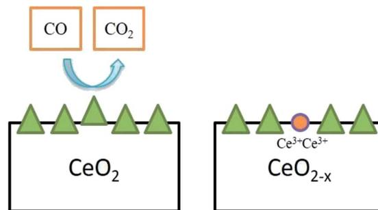
Fig. 4 Oxygen vacancy created by  $\text{CeO}_2$  particle while oxidizing CO to  $\text{CO}_2$ , and two  $\text{Ce}^{4+}$  atoms were reduced simultaneously (adapted from K. Reed *et al.*, *Environ. Sci.: Nano*, The Royal Society of Chemistry, 2014 (ref. 22)).
