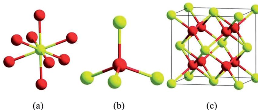
Fig. 2 Structurally analyzed ceria crystals  $\text{Ce}_4\text{O}_8$  (unit cell); in (a) and (b) yellow color represents eight-folds of cerium atoms and red represents four-fold oxygen atoms in ceria crystal structure; (c) is the basic fcc fluorite lattice structure of  $\text{Ce}_4\text{O}_8$  (reproduced from K. Reed *et al.*, *Environ. Sci.: Nano*, The Royal Society of Chemistry, 2014 (ref. 22)).
