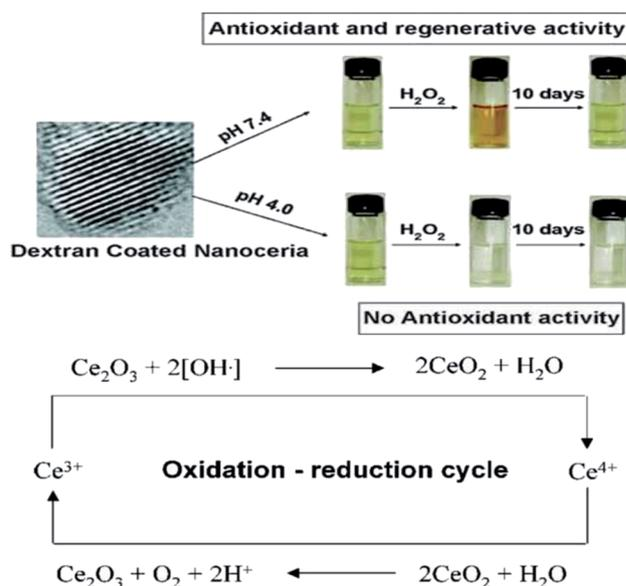
Fig. 7 Top: Color change in solutions of cerium oxide nanoparticle coated with dextran at basic and acidic pH environment on addition of H<sub>2</sub>O<sub>2</sub>. Bottom: Detailed probable revised mode of mechanism data cerium oxide nanoparticle auto-regenerative attribute and free-radical scavenging property (reproduced from J. M. Perez *et al.*, *Small*, John Wiley and Sons, 2008 (ref. 106)).
