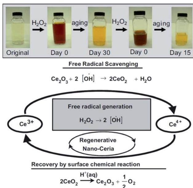
Fig. 6 Top: Observation of change in color when, cerium oxide nanoparticle coated with dextran was treated with H<sub>2</sub>O<sub>2</sub> at different time intervals. Bottom: Schema of chemical reaction showing auto-regenerative properties cerium oxide nanoparticles and possible mode of mechanism data of the cerium oxide nanoparticle autocatalytic behavior and free-radical scavenging property (reproduced from M. Das *et al.*, *Biomaterials*, Elsevier, 2007 (ref. 105)).
