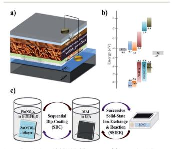
Fig. 1 Description of (a) PHJ PrSC structure, (b) energy level diagram, and (c) the preparation of the MAPbl $_3$  perovskite films by sequentially dip-coating a ZnO-covered c-TiO $_2$ /FTO substrate in aqueous Pb(NO $_3$ ) $_2$  and MAI solutions.
