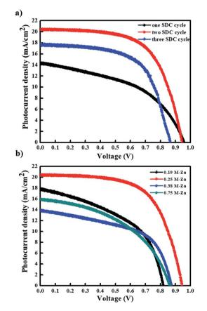
Fig. 7 Current–voltage (J-V) curves under AM 1.5 irradiation (100 mW cm $^{-1}$ ) for the PHJ PrSCs based on (a) MAPbI $_3$  perovskite layers fabricated by the designated number of SDC cycles followed by three SSIER cycles on ZnO (0.25 M-Zn) over the c-TiO $_2$  layers, and (b) MAPbI $_3$  perovskite layers fabricated on ZnO (0.19 M-Zn), ZnO (0.25 M-Zn), ZnO (0.38 M-Zn), and ZnO (0.75 M-Zn) over the c-TiO $_2$  layers under two SDC cycles.
