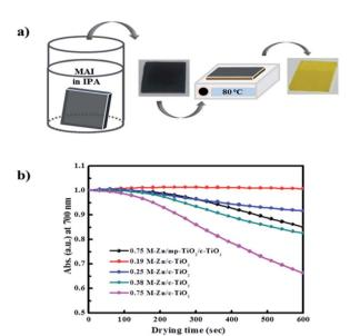
Fig. 3 (a) The decomposition behaviors and (b) the decrease in the absorbance at 700 nm over 600 s of the MAPbl<sub>3</sub> perovskite film fabricated by this sequential dip-coating deposition on ZnO/c-TiO<sub>2</sub> layer observed during solvent drying.
