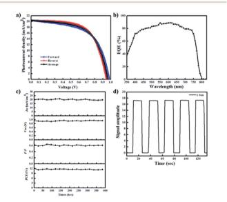
Fig. 8 (a) The hysteresis of the J-V curves in both scan directions under AM 1.5 irradiation (100 mW cm $^{-1}$ ), (b) EQE spectra, (c) stability, and (d) photoswitching phenomenon for the most efficient PHJ PrSCs fabricated using dip-coating deposition approach on the thin ZnO/c-TiO<sub>2</sub> bilayer ETL under two SDC cycles.
