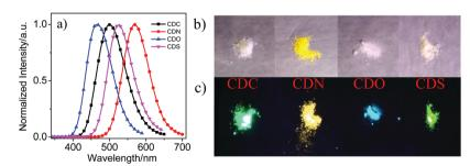
Fig. 3 (a) The normalized emission spectra of CDC, CDN, CDO and CDS in the solid state,  $\lambda_{\rm ex}=300$  nm for CDC and CDO,  $\lambda_{\rm ex}=330$  nm for CDN and CDS. (b) Photos of compounds CDC, CDN, CDO and CDS as solid powders under room light and (c) fluorescence images under UV illumination (365 nm), 20 °C.
