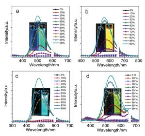
Fig. 2 Fluorescence spectra of (a) CDC, (b) CDC, (c) CDF and (d) CDS in THF/water mixtures with different water volume fractions;  $\lambda_{ex}$  = 300 nm for **CDC** and **CDO**,  $\lambda_{ex}$  = 330 nm for **CDN** and **CDS**, c = 5.0  $\times$  10<sup>-5</sup> M, 20  $^{\circ}$ C (light scattering from the incident light was omitted in the spectra).
