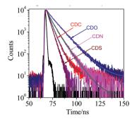
Fig. 5 Emission decay profiles of CDC, CDN, CDO and CDS in the solid state,  $\lambda_{ex}$  = 340 nm, 20 °C.
