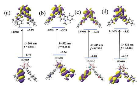
Fig. 9 Frontier molecular orbitals in the first singlet excited state (S<sub>1</sub>) optimized geometries of (a) CDC, (b) CDN, (c) CDO and (d) CDS in the gas state and the lowest-energy electronic transitions from the TD-DFT calculation at the B3LYP/6-31G(d,p) level by Gaussian 09.
