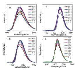
Fig. 4 The PL spectra of (a) CDC, (b) CDN, (c) CDO and (d) CDS in the solid state during cooling from 333 to 77 K,  $\lambda_{\rm ex}$  = 300 nm for **CDC** and CDO,  $\lambda_{ex}$  = 330 nm for CDN and CDS.
