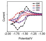
Fig. 7 Cyclic voltammogram of CDC, CDN, CDO and CDS,  $c = 1.0 \times$  $10^{-3}$  M. The deaerated acetonitrile solution contained the compounds, 0.10 M  $Bu_4NPF_6$  as supporting electrode,  $Ag/AgNO_3$  as a reference electrode, scan rates: 100 mV s<sup>-1</sup>. For all compounds, ferrocene (Fc) (c =  $1.0 \times 10^{-3}$  M) was used as an internal reference, 20 °C.
