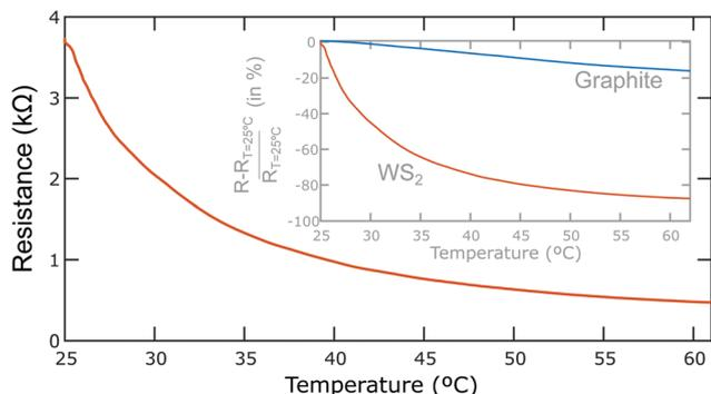
**Fig. 4** Temperature dependence of the resistance of WS<sub>2</sub>-on-paper thermoresistive devices. (a) Resistance vs. temperature for a WS<sub>2</sub>-on-paper device with pencil-drawn interdigitated devices. (inset) Comparison between the resistance vs. temperature curves measured for the WS<sub>2</sub> and a graphite thermoresistive devices on paper.
