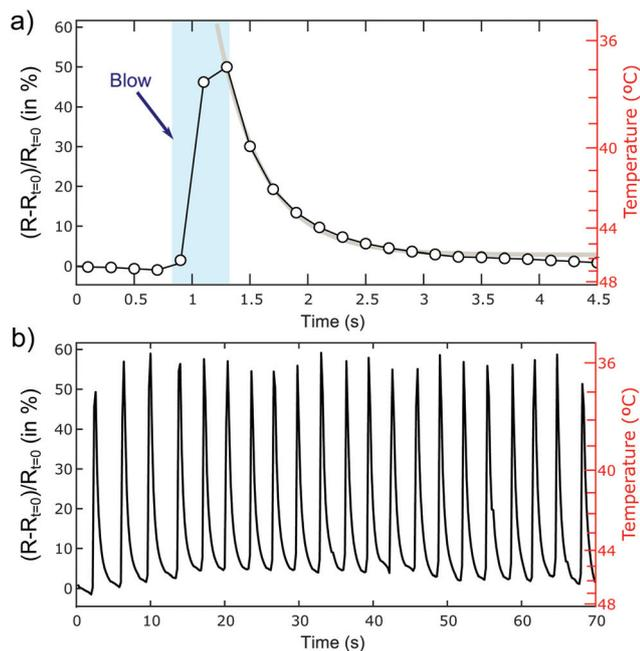
**Fig. 5** Response time of WS<sub>2</sub>-on-paper thermoresistive devices upon sudden temperature changes. (a) Resistance change vs. time of a WS<sub>2</sub>-on-paper device subjected to a sudden change in temperature. The device is warmed up to ~45 °C and at time  $t \sim 1$  s a hand pump blows cool air onto the device. (b) 21 breathing cycles to demonstrate the reproducibility of the thermoresistive device.
