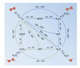
Fig. 2 Possible reduction pathways from O2 to H2O (blue) and oxidation pathways from H<sub>2</sub>O to O<sub>2</sub> (green). The black arrows denote the adsorption and desorption/diffusion of species from the bulk solution and the catalyst. Oxygen and hydrogen atoms are represented as red and white balls, respectively. Stoichiometric H<sub>2</sub>O is omitted for clarity.<sup>28</sup>
