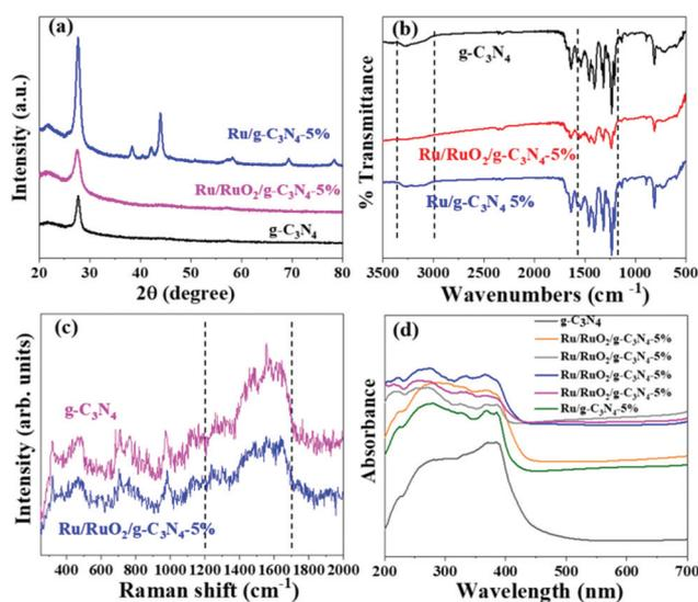
Fig. 1 XRD patterns (a), FTIR spectra (b), Raman spectra (c), and UV-Vis spectra (d) of  $g\text{-C}_3\text{N}_4$ ,  $\text{Ru}/\text{RuO}_2/g\text{-C}_3\text{N}_4\text{-}5\%$  and  $\text{Ru}/g\text{-C}_3\text{N}_4\text{-}5\%$ .
