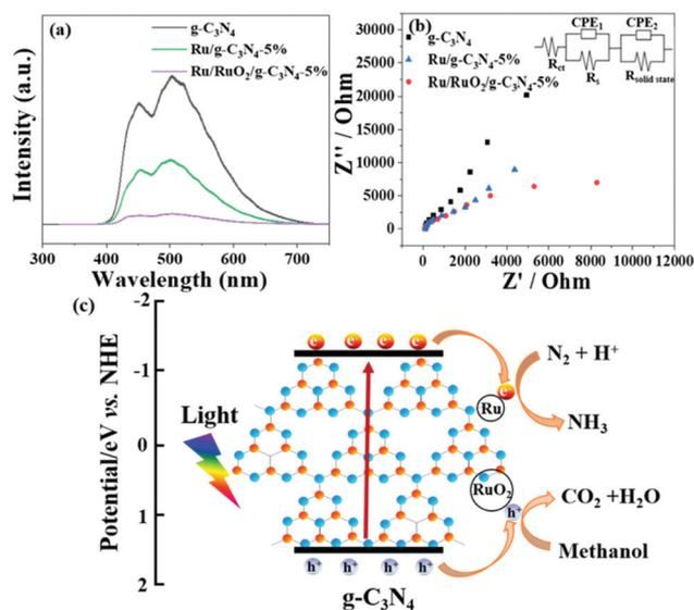
**Fig. 5** The photoluminescence (a) and EIS (b) of Ru/RuO<sub>2</sub>/g-C<sub>3</sub>N<sub>4</sub>-5% and g-C<sub>3</sub>N<sub>4</sub> (inset is the interface charge transfer by fitting the impedance plots). A potential mechanism for the ammonia photosynthesis activity of Ru/RuO<sub>2</sub>/g-C<sub>3</sub>N<sub>4</sub>-5% (c).
