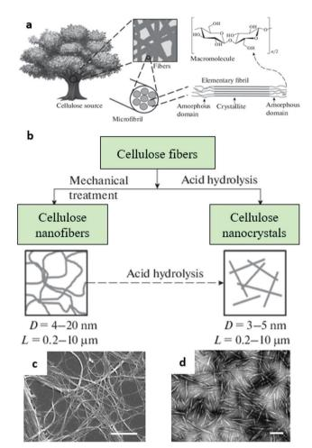
Fig. 7 (a) Hierarchical structure of cellulose and (b) synthesis of cellulose nanofibers and cellulose nanocrystals; adopted from ref. 143, copyright@ 2018, Springer Nature. (c and d) SEM images of cellulose NFs and CNCs, respectively. (c) Adopted from ref. 144, copyright © 2013, Springer Nature. (d) Adopted from ref. 145, copyright @ 2008, Royal Society of Chemistry.
