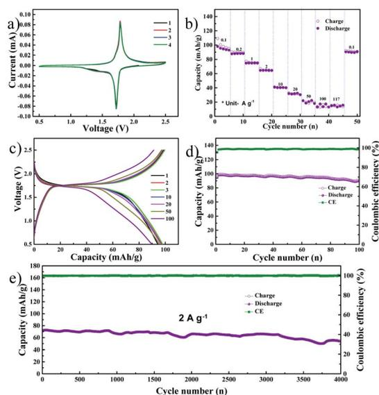
Fig. 3 (a) Results of CV tests conducted on the symmetric NVP cell in the DME electrolyte at a scan rate of  $0.1 \text{ mV s}^{-1}$  in the 0.5 V to 2.5 V voltage window. (b) Results of rate performance tests conducted on the symmetric cell. (c) Voltage profile and (d) the corresponding cycling performance at a current density of  $0.1 \text{ A g}^{-1}$ . (e) Cycling performance at a current density of  $2 \text{ A g}^{-1}$ .
