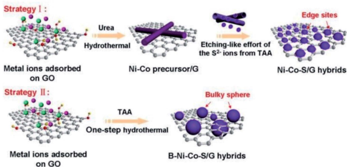
Fig. 6 Schematic illustrations of the in situ formation of the integrated edge site-enriched Ni–Co–S/G hybrid architectures (Strategy I), fabricated by the Kirkendall effect-involved anion exchange reaction of the NiCo-precursor on graphene with abundant S^{2-} ions derived from TAA. The B–Ni–Co–S/G hybrids were directly fabricated via a one-step hydrothermal method (Strategy II). 99
