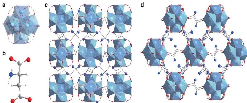
Fig. 2 Crystal structures of MIP-202(Zr). (a) The 12-connected  $Zr_6(\mu_3-O)_4(\mu_3-OH)_4(COO^-)_{12}$  cluster SBU. (b) The aspartic acid linker. (c and d) The structure of MIP-202(Zr) viewed along the  $a$ -axis (c) and the (101) plane (d). Zr atoms or polyhedra, oxygen, carbon, nitrogen, and hydrogen atoms are respectively shown with colors of light blue, red, gray, dark blue, and white. Reproduced from ref. 39 with permission from Nature Publishing Group.
