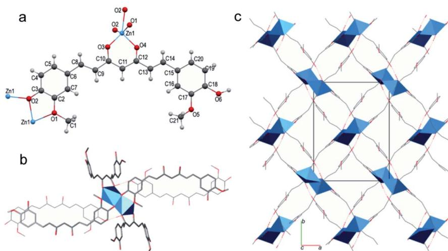
Fig. 6 The structure of sc-CCMOF-1: (a) the coordination mode; (b) the  $Zn_2O_8$  SBU structure and (c) the 2D framework. Reproduced from ref. 54 with permission of American Chemical Society.
