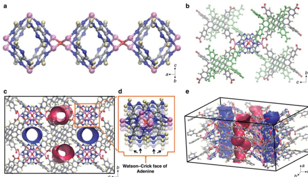
**Fig. 1** Structural simulation of SION-19. (a) and (b) Three-dimensional structures of SION-19 at different scales, where pink represents Zn atoms, red represents O atoms, blue represents N atoms, gray represents C atoms, and yellow represents H atoms. (c–e) The pore structure of SION-19. (d) Watson–Crick surface provided by Ade. Reproduced from ref. 29 with permission from Nature Publishing Group.
