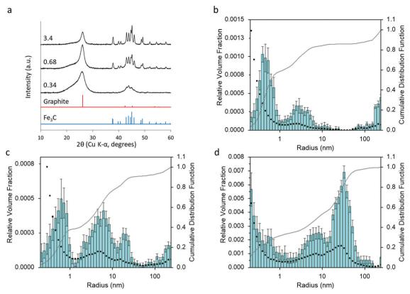
Fig. 6 (a) PXRD data for carbon samples prepared from starch (5 g) with various amounts (mmol) of iron nitrate, held at 800  $^{\circ}$ C for 1 h. Particle size histograms coupled with visibility limits (black dots, left *y*-axis) and cumulative distribution functions (right *y*-axis) for carbons from starch (5 g) with (a) 3.4, (b) 0.68 and (c) 0.34 mmol of iron nitrate.
