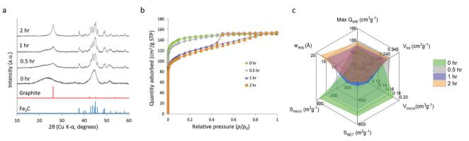
Fig. 7 (a) XRD diffraction patterns for carbons synthesized from starch (5 g) and iron nitrate (3.4 mmol) and held at 800 °C for different times. (b) N<sub>2</sub> adsorption isotherms and (c) adsorptive characteristics of these starch-derived carbons.
