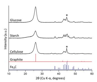
Fig. 2 PXRD patterns for carbon/Fe $_3$ C samples produced from glucose, starch and cellulose (5 g) and iron nitrate (0.68 mmol), held at 800 °C for 1 h. (\*) indicates presence of minor  $\alpha$ -Fe phase.
