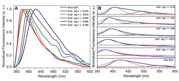
Fig. 10 (A) Photoluminescence spectra (in the solid state) and (B) deconvolution of the spectra of pure ZnO and different sets of ZnO-Aq microstructures
