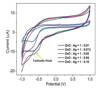
Fig. 9 Cyclic voltammograms of different sets (0.01 M) of Ag/ZnO microstructures.
