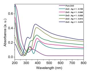
Fig. 3 Diffuse reflectance spectra of pure ZnO and different sets of Ag/ ZnO microstructures
