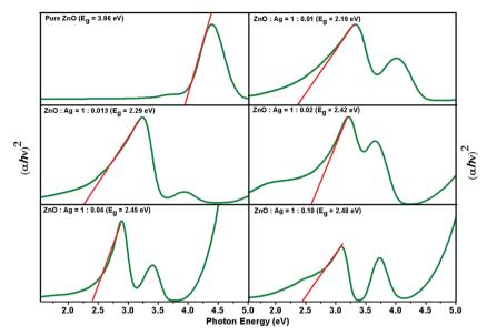
Fig. 4 Tauc plot for the estimation of the band gap energy of pure ZnO and different sets of Ag/ZnO microstructures.
