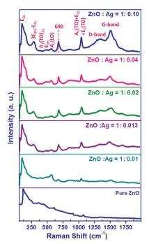
Fig. 8 Raman spectra of pure ZnO and different sets of Ag/ZnO microstructures.
