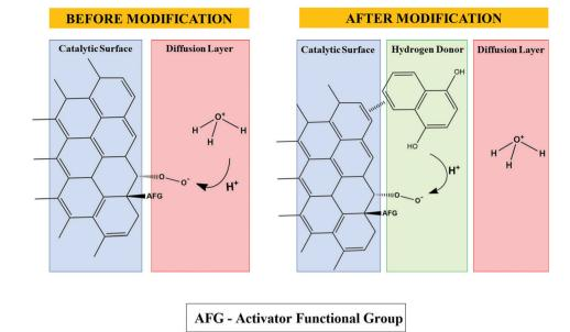
Fig. 2 Proposed scheme for the unmodified carbon surface and incorporation of the organic compound 1,4-naphthoquinone, which acts as an H<sup>+</sup> donor for the ORR.
