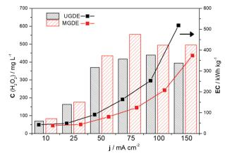
Fig. 4 Comparison of the maximum concentration of H<sub>2</sub>O<sub>2</sub> electrogenerated in 120 min on the unmodified GDE (UGDE) and modified GDE (MGDE) with the respective energy consumption for the - ■ - UGDE and — ■ — MGDE, calculated based on eqn (10).
