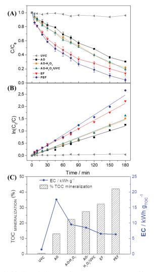
**Fig. 5** (A) Effect of different AEOPs on PRM degradation in 180 min of experiment at  $j=75~\text{mA}~\text{cm}^{-2}$  using the 1.0% NQE modified GDE with 0.1 mol L<sup>-1</sup> K<sub>2</sub>SO<sub>4</sub> under pH 2 and 0.2 bar of O<sub>2</sub> flow; (B) analysis of the pseudo-first order kinetics; and (C) comparison between the TOC mineralization and energy consumption in each system.
