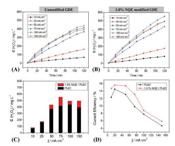
**Fig. 3** (A) Electrogenerated  $H_2O_2$  concentration at different current densities on the unmodified GDE and (B) on the 1.0% NQE modified GDE; (C) comparison of the maximum concentration obtained in 120 minutes of electrosynthesis; and (D) current efficiency of all the densities investigated in 0.1 mol  $L^{-1}$  K<sub>2</sub>SO<sub>4</sub> electrolyte, pH = 2.5 (H<sub>2</sub>SO<sub>4</sub>) under 0.2 bar O<sub>2</sub> pressure.
