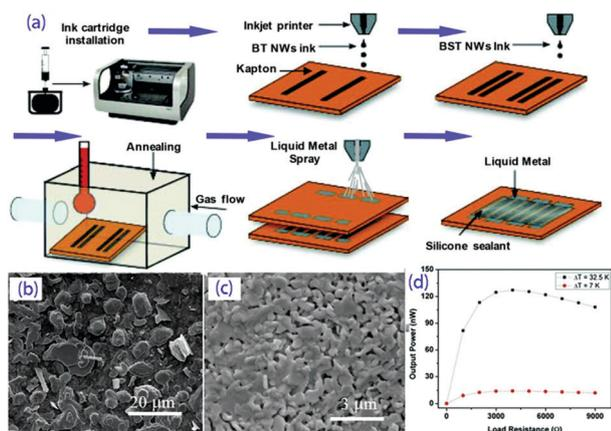
Fig. 8 (a) Fabrication schematic for the development of the inkjet-printed TEG device; SEM micrographs of the printed BST50 (b) and BT50 (c) nanowires annealed at  $450^\circ\text{C}$  for 10 min; (d) output power of the printed TEG as a function of load resistance. (Reproduced from ref. 103 with permission from The Royal Society of Chemistry.)
