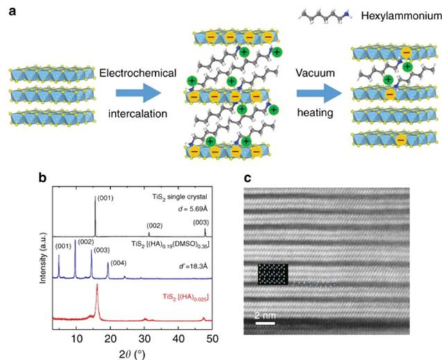
Fig. 2 (a) Schematic of the electrochemical intercalation process. (b) XRD patterns of  $\text{TiS}_2$  single crystal and its related superlattice structures. (c) Magnified STEM image of  $\text{TiS}_2[(\text{HA})_{0.025}]$ . (Reproduced from ref. 33 with permission from Nature Communication.).
