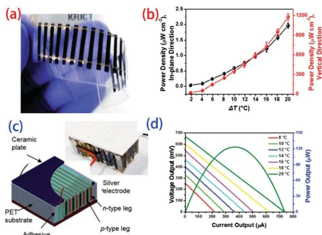
**Fig. 15** Fabrication of planar (a) and vertical (c) thermoelectric modules and power densities as a function of temperature gradient for the (b) planar and (d) vertical modules. (Reproduced from ref. 129 with permission from The Royal Society of Chemistry.).
