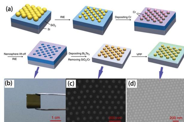
**Fig. 9** (a) Scheme of the fabrication of the organic/inorganic hybrid film *via* nanosphere lithography, (b) digital photograph of closely packed monolayer PS nanospheres on a SiO<sub>2</sub>/Si substrate after etching, SEM image of (c) Bi<sub>2</sub>Te<sub>3</sub> nanoparticle arrays prepared by using 100 nm PS nanospheres as patterns and (d) PEDOT/Bi<sub>2</sub>Te<sub>3</sub>(100) hybrid films.<sup>109</sup>
