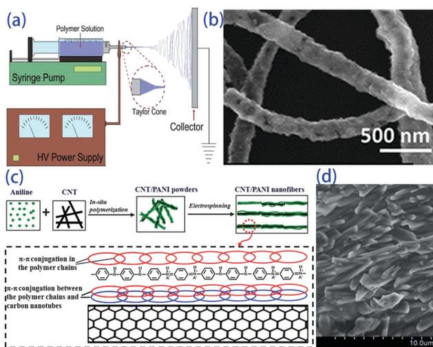
Fig. 4 (a) Scheme of a conventional electrospinning setup,<sup>39</sup> (b) electro-spun hollow  $\text{PbTe}$  nanofibers,<sup>44</sup> (c) schematic of the formation mechanism and (d) SEM image of CNT/PANI nanofibers.<sup>45</sup>
