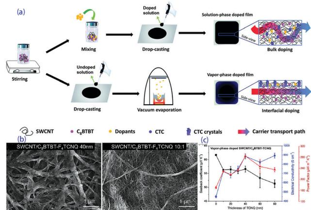
Fig. 11 (a) Fabrication processes of the composite films by bulk doping or interfacial doping, (b) SEM pictures of an SWCNT/C<sub>8</sub>BTBT-F<sub>4</sub>TCNQ film obtained with a vapor-phase process and an SWCNT/C<sub>8</sub>BTBT-F<sub>4</sub>TCNQ film obtained with a solution-phase process, and (c) the transport properties of vapor-phase doped SWCNT/C<sub>8</sub>BTBT-TCNQ with different thicknesses of TCNQ.<sup>145</sup>
