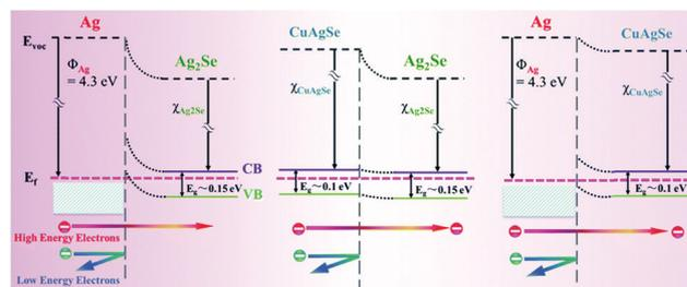
Fig. 3 Equilibrium band diagrams for  $\text{Ag}/\text{Ag}_2\text{Se}$ ,  $\text{CuAgSe}/\text{Ag}_2\text{Se}$  and  $\text{Ag}/\text{CuAgSe}$ .<sup>38</sup>
