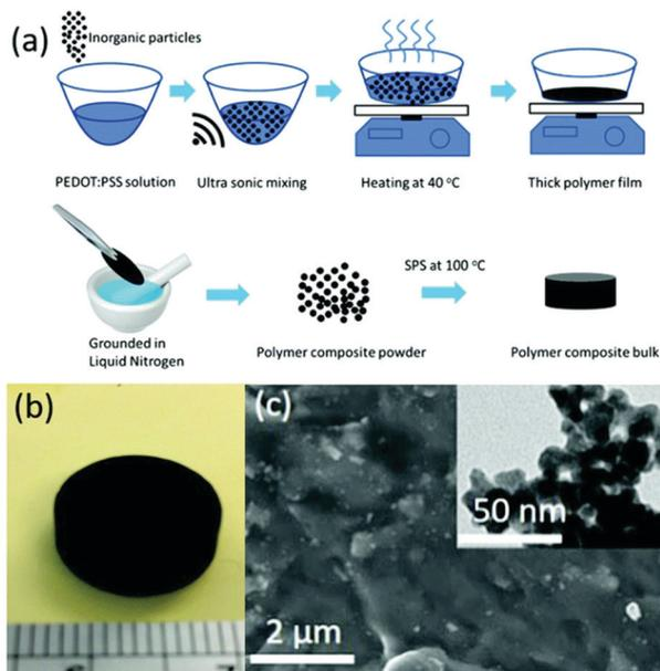
Fig. 5 (a) Process used to synthesize bulk polymers. (b) Photograph of a polymer bulk sample after applying SPS. (c) CSS polymer bulk with an inset showing a TEM image of  $\text{Cu}_2\text{SnSe}_3$  nanoparticles. (Reproduced from ref. 56 with permission from The Royal Society of Chemistry.)
