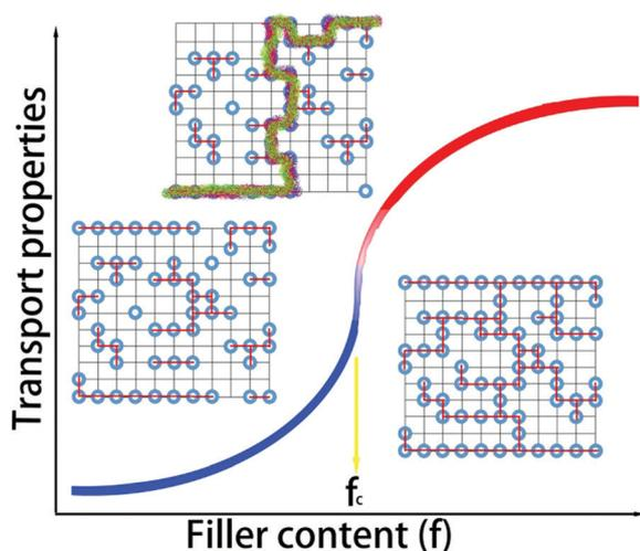
Fig. 1 Percolation theory and nonlinear changes in the transport properties of composites near the percolation threshold  $f_c$  (dashed blue line). The insets show the geometric phase transition of fillers (denoted by dark spots) in the microstructures of the composites near percolation.
