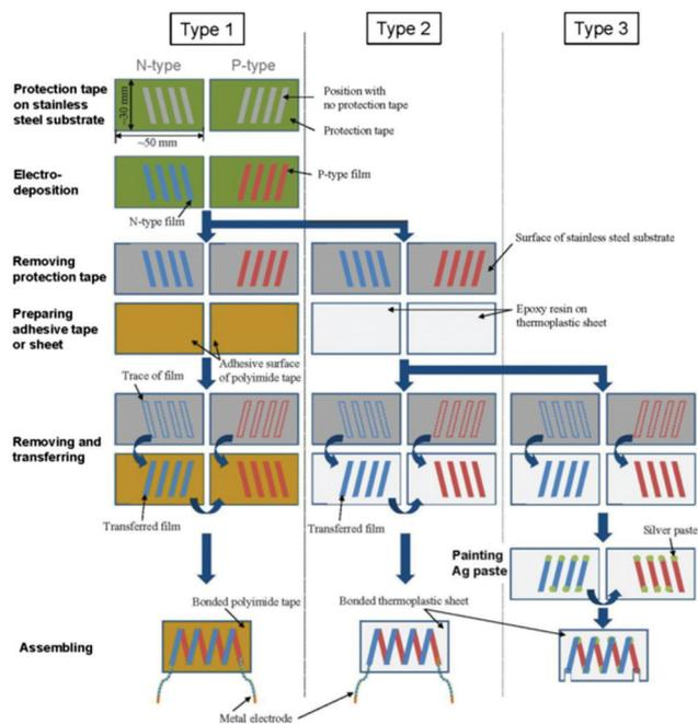
**Fig. 14** Schematic process, flow diagram and photographs of the three types of flexible thin-film TEGs.<sup>73</sup>
