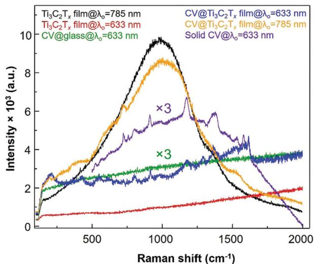
Fig. 5 The normal Raman spectra (ca.  $12.732 \text{ ng cm}^{-2}$  of CV on bare glass and solid CV) and surface-enhanced Raman scattering (SERS) of CV dye molecules (ca.  $12.732 \text{ ng cm}^{-2}$ ) adsorbed on  $\text{Ti}_3\text{C}_2\text{T}_x$  film@glass with excitation laser wavelengths of both 633 nm and 785 nm.
