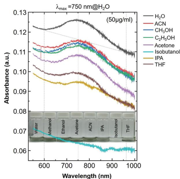
Fig. 2 The UV-visible NIR spectra of colloidal solutions of delaminated  $\text{Ti}_3\text{C}_2\text{T}_x$ –MXene ( $d\text{-Ti}_3\text{C}_2\text{T}_x$ ) flakes dispersed in various organic solvents. A photograph of diluted  $d\text{-Ti}_3\text{C}_2\text{T}_x$  solution ( $50 \mu\text{g ml}^{-1}$ ) in various organic solvents is presented in the inset.
