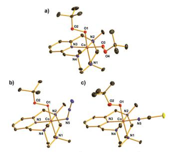
Fig. 2 ORTEP plots of the (a)  $Co^{III}-(OO^tBu)_2$  complex,  $[Co^{III}(Me_3-TPADP)(OO^tBu)_2]^+$  (2), and  $Co^{III}-(OO^tBu)(X)$  complexes,  $[Co^{III}(Me_3-TPADP)(OO^tBu)(X)]^+$  (X = (b)  $N_3$  (4), (c) NCS (5)), with thermal ellipsoids drawn at the 30% probability level. Hydrogen atoms are omitted for clarity.
