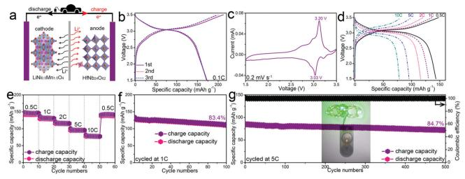
$\textbf{Fig. 3} \hspace{0.2cm} \textbf{(a)} \hspace{0.2cm} \hspace{$ (b) initial three-cycle charging/discharging curves at 0.1C, (c) CV at 0.2 mV s<sup>-1</sup>, (d) charging/discharging curves at different current rates, (e) rate performance, and cyclability at (f) 1C and (g) 5C (inset: green LED lit up by the full cell).
