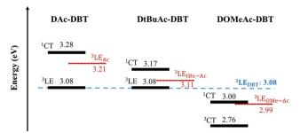
**Fig. 6** A schematic energy diagram of **DAc-DBT**, **DtBuAc-DBT** and **DOMeAc-DBT**. All energies are given in eV and were calculated from the onsets of the corresponding spectra in zeonex films, compared with their individual D and A moieties. No indication of <sup>3</sup>CT states is obtained in **DAc-DBT** and **DtBuAc-DBT** from calculations, neither are they observed in our experiments, therefore, their <sup>3</sup>CT states are not represented in this diagram.
