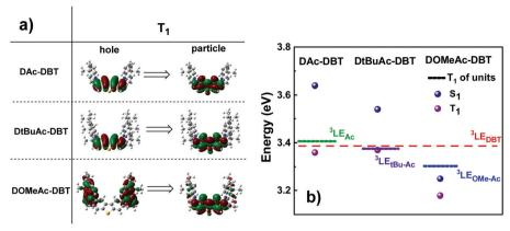
Fig. 4 (a) Natural transition orbitals (NTO) corresponding to the first triplet transitions and (b) singlet and triplet energy diagram of **DAc-DBT**, **DtBuAc-DBT** and **DOMeAc-DBT** along with the energy levels of the individual units (TD-DFT rBMK/6-31G(d)). Hole refers to the highest occupied natural transition orbital (HONTO), while particle refers to lowest unoccupied natural transition orbital (LUNTO).<sup>57</sup>
