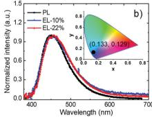
Fig. 9 (a) EQE vs. luminance characteristics. Inset shows the device structure and energy levels. (b) The comparison of PL spectrum of DPEPO:10%DtBuAc-DBT film and EL spectra of 10% and 22% doping concentration in blue devices collected at 9 V. The inset shows the CIE coordinates of the devices.
