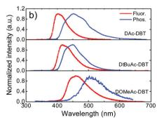
Fig. 5 (a) UV-vis absorption and fluorescence spectra of **DAc-DBT**, **DtBuAc-DBT** and **DOMeAc-DBT** in toluene solutions  $(1.0 \times 10^{-4} \text{ M})$  measured at room temperature. (b) Steady-state fluorescence collected at room temperature and time-resolved phosphorescence spectra collected with delay time of 56 ms at 80 K for the three molecules in zeonex films (1 wt). Excitation at 355 nm.
