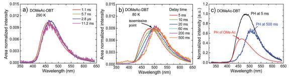
Fig. 8 DOMeAc-DBT in zeonex film: time-resolved area normalized emission spectra at (a) 290 K and (b) 80 K. (c) Phosphorescence spectra recorded at delay times of 5 ms and 500 ms, compared with the that of the donor OMe-Ac unit measured at 80 K.
