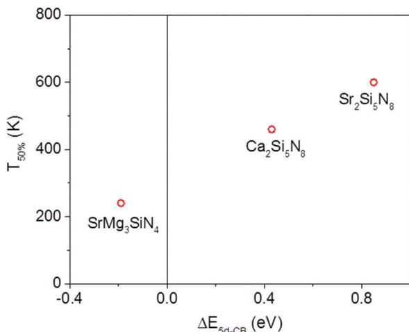
Fig. 5 Temperature at which 50% of the  $\text{Eu}^{2+}$  5d–4f emission is quenched ( $T_{50\%}$ ) versus the energy difference ( $\Delta E_{5d\text{-CB}}$ ) between the bottom of the host lattice conduction band and the lowest relaxed  $\text{Eu}^{2+}$  5d state for  $\text{SrMg}_3\text{SiN}_4\text{:Eu}^{2+}$ ,  $\text{Ca}_2\text{Si}_5\text{N}_8\text{:Eu}^{2+}$  and  $\text{Sr}_2\text{Si}_5\text{N}_8\text{:Eu}^{2+}$ .
