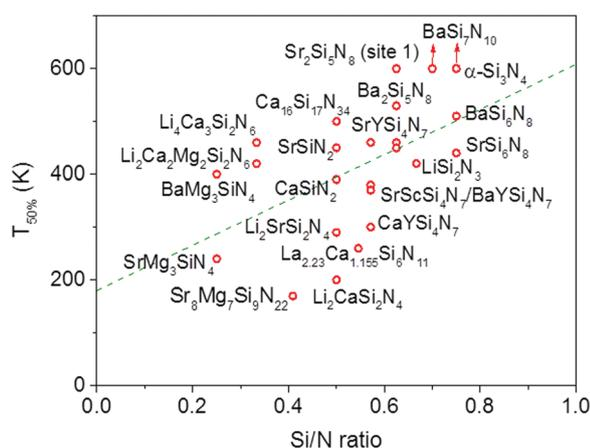
Fig. 4 Temperature at which 50% of the  $\text{Eu}^{2+}$  5d–4f emission is quenched ( $T_{50\%}$ ) versus the Si/N ratio of the  $\text{Eu}^{2+}$  doped nitridosilicates. The dashed green lines is a linear fit through the data points to indicate the trend.
