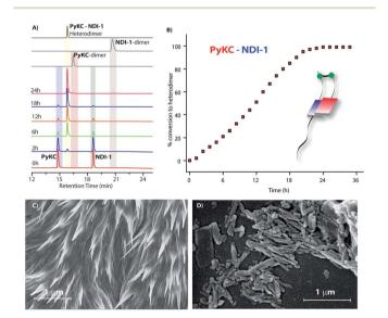
Fig. 3 (A) Time dependent chromatograms showing the exclusive formation of the PyKC-NDI-1 heterodimer using the present protocol. (B) % conversion to the heterodimer with time as obtained from (A). (C) and (D) FESEM images of the freeze dried samples obtained from the combinations of NDI-1 with (C) PyK<sup>D</sup>C and (D) Py1KC.
