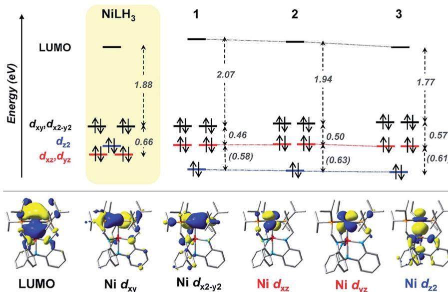
Fig. 6 (Top) MO diagrams of NiLH<sub>3</sub> and complexes 1–3. The ligand field energies (in eV) are based on UV-Vis data (Table 5). TD-DFT calculated energies are shown (in eV, italicized within parentheses) when experimental values were not obtainable. (Bottom) MOs for complex 2, which are representative of those for the series. Note that MO energies are drawn to scale, but energy comparisons across the complexes are qualitative.
