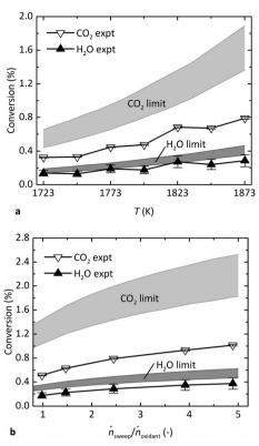
Fig. 4 Comparison of the average experimental conversion of CO<sub>2</sub> and H<sub>2</sub>O at steady state versus equilibrium limits as a function of (a) T, at  $\dot{n}_{\text{sweep}}/\dot{n}_{\text{oxidant}}$  = 2.4 and 1 Pa O<sub>2</sub>, and (b)  $\dot{n}_{\text{sweep}}/\dot{n}_{\text{oxidant}}$ , at 1873 K and 0.5 Pa O2.
