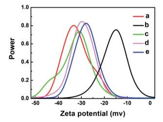
Fig. 3 Zeta potential graphs of: (a) GO, (b) Ag, (c) GO-Ag, (d) GO-TiO2@ZnO, and (e) GO-Ag-TiO2@ZnO in water.
