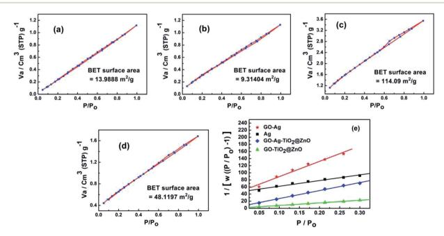
Fig. 5  $N_2$  adsorption/desorption isotherm curve of (a) Ag, (b) GO-Ag, (c) GO-TiO<sub>2</sub>@ZnO, and (d) GO-Ag-TiO<sub>2</sub>@ZnO nanocomposites. (e) Langmuir fits from the  $N_2$  adsorption data for Ag, GO-Ag, GO-TiO<sub>2</sub>@ZnO, and GO-Ag-TiO<sub>2</sub>@ZnO nanocomposites.
