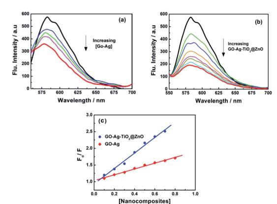
Fig. 8 Fluorescence quenching of ctDNA with different concentrations of (a) GO-Ag and (b) GO-Ag-TiO<sub>2</sub>@ZnO in Tris-HCl buffer;  $\lambda_{ex} = 260 \text{ nm}$ ; (c) Stern-Volmer plots.
