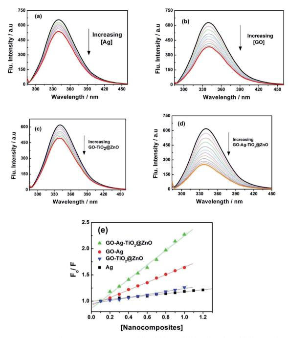
Fig. 7 Fluorescence spectra of BSA with different concentration of (a) Ag, (b) GO-Ag, (c) GO-TiO<sub>2</sub>@ZnO, and (d) GO-Ag-TiO<sub>2</sub>@ZnO at  $\lambda_{ex}$  = 280 nm. (e) Stern-Volmer plots.
