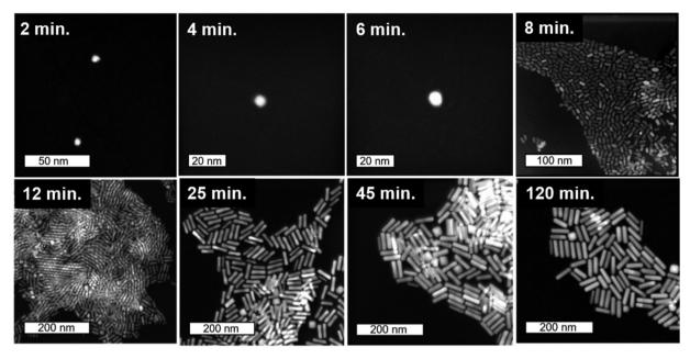
Fig. 2 Timecourse STEM images. Starting from 2 nm Au seeds, STEM images taken from colloidally synthesized Au nanorods quenched with BSPP at time points from 2 minutes into growth (top-left) to final product nanorods (bottom-right). The first three images are collected using cryo-STEM (see ESI† for details).
