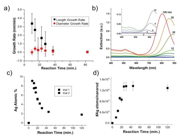
Fig. 3 Nanoparticle growth and composition. (a) EM determined length and diameter growth rates as a function of reaction time, (b) UV-vis spectra as a function of reaction time; inset shows a magnified view of early time point spectra, (c) XRF-determined nanoparticle composition and (d) XRF and EM determined number of Ag atoms per nanorod.
