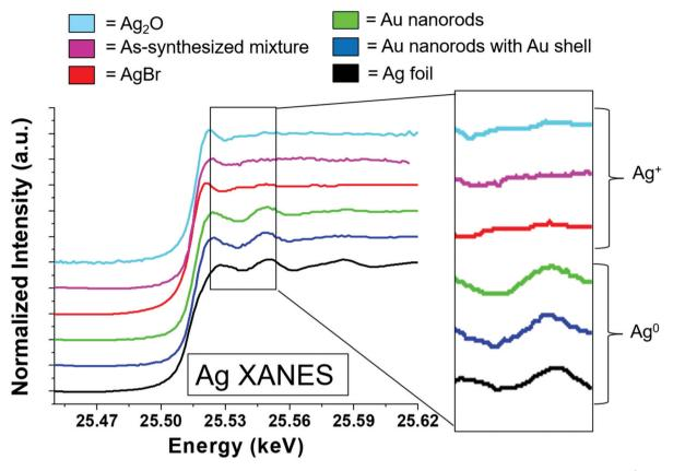
Fig. 4 Ag K-edge XANES data from 120 min final product nanorods (middle, green) compared to standards with Ag<sup>+</sup> (top 3) and Ag<sup>0</sup> (bottom 2). A blowup of the near edge region is shown on the right-hand-side for each spectrum.
