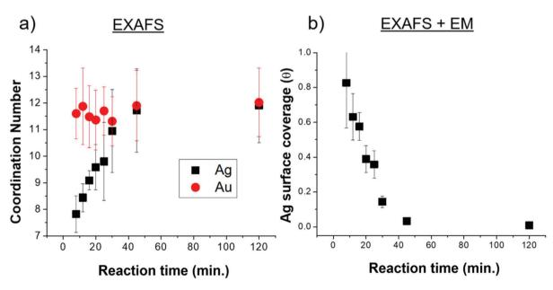
Fig. 5 Ag coordination number and surface coverage. (a) Coordination numbers extracted from Ag K and Au L3 edge XAFS spectra. (b) Ag surface coverage, extracted from a combination of XAFS-extracted coordination numbers, EM-determined dimensions and the assumption that Ag on the surface has a CN of 7.
