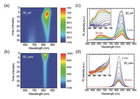
Fig. 6 Photostability of the reference and converted 3D FAPbl<sub>3</sub> perovskite films. (a) 2D pseudo-color plot of the PL spectra of the reference film as a function of continuous laser excitation time. (b) 2D pseudo-color plot of the PL spectra of the converted film as a function of continuous laser excitation time. (c) Evolution of the PL spectra of the reference film. (d) Evolution of the PL spectra of the converted film.
