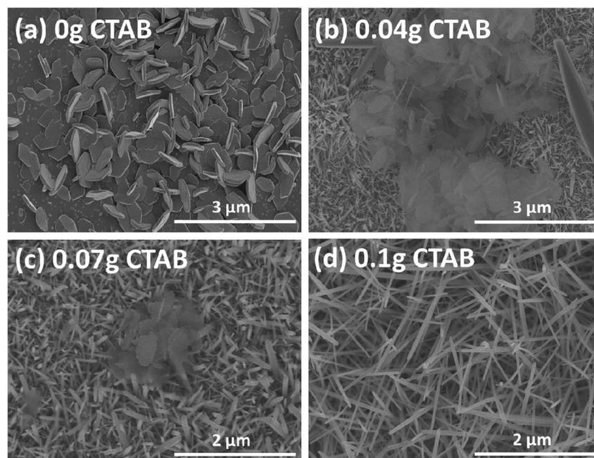
Fig. 1 Plane-view SEM micrographs of the PbI<sub>2</sub> micro-needles synthesized by the hydrothermal route with various amounts of CTAB: 0 g (a), 0.04 g (b), 0.07 g (c), and 0.10 g (d), respectively.
