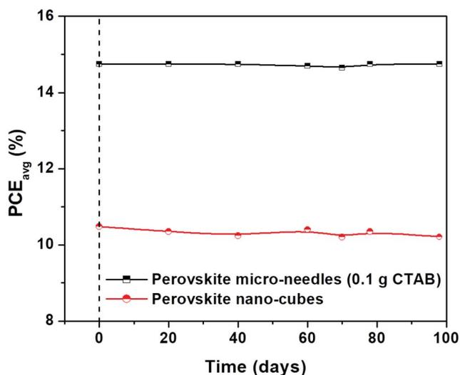
Fig. 6 Long-term stability test of un-encapsulated devices based on MAPbI<sub>3</sub> micro-needles and perovskite nano-cubes stored in dry air.
