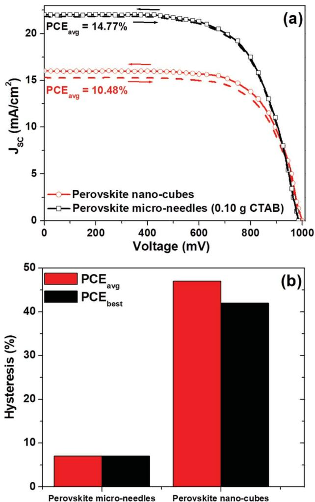
Fig. 4 (a) Comparison of  $J$ - $V$  plots of perovskite devices based on MAPbI<sub>3</sub> micro-needles and nano-cubes, and (b) hysteresis for devices with MAPbI<sub>3</sub> micro-needles and nano-cubes, respectively.
