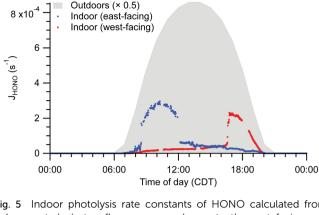
Fig. 5 Indoor photolysis rate constants of HONO calculated from solar spectral photon fluxes measured near to the east-facing and west-facing windows under clear sky conditions. Photon fluxes were determined from measured spectral irradiance. Outdoor HONO photolysis rate constants based on tropospheric ultraviolet and visible (TUV) radiation model results are shaded in grey for comparison.<sup>64</sup>
