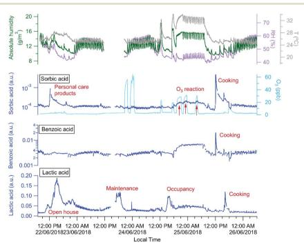
Fig. 10 Three organic acids – sorbic, benzoic, and lactic acid – varied during four days of the campaign (open house, maintenance, occupancy, and layered day) with temperature in grey, relative humidity/RH in purple, and absolute humidity/AH in dark green. Cooking or food sources of all three organic acids are apparent, as are occupant emissions of lactic acid and personal care product sources of sorbic acid.
