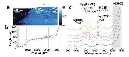
Fig. 11 (a) 3-D AFM height image of a deposition on window glass from a stir-fry event. (b) Height profile from the purple line shown in panel (a) and (c) IR spectra taken at the corresponding colored markers in panels A and B.
