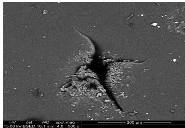
Fig. 12 A commonly encountered result of electrical breakdown in silicone elastomers is a macroscopic mechanical failure, whereby the thin elastomer film is completely torn apart. The picture shows dielectric breakdown in a film which was under small load only. It leads to a microscopic pinhole, which then may propagate mechanical failure. The presence of enhanced local stresses at the cracks around the breakdown zone, which is solidified to some extent, leads to tear propagation and usually also complete film failure. Reproduced from ref. 14 with permission from the Technical University of Denmark (DTU), copyright 2017.
