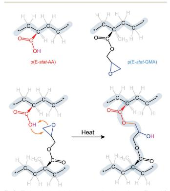
Fig. 2 The branched statistical ethylene–acrylic acid copolymer p(E-stat-AA) and ethylene–glycidyl methacrylate copolymer p(E-stat-GMA) used in this study. At the bottom, the reaction scheme for p(E-stat-AA) with p(E-stat-GMA).
