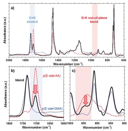
Fig. 3 (a) ATR-FTIR spectrum of the p(E-stat-AA):p(E-stat-GMA) polymer blend at stochiometric ratio; (b) reduction of the C=O stretching peak at 1705 cm<sup>-1</sup> upon blending; (c) reduction of the O-H out-of-plane bend peak at 940 cm<sup>-1</sup> upon blending; all spectra are normalized and p(E-stat-AA) and p(E-stat-GMA) intensities are scaled to their respective concentration in the blend; blend (solid); p(E-stat-AA) (dashed); p(E-stat-GMA) (dotted).
