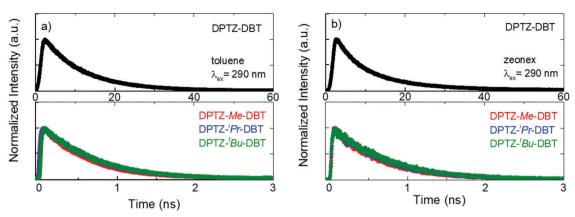
Fig. 5 Emission decays of DPTZ-DBT, DPTZ-Me-DBT, DPTZ-iPr-DBT and DPTZ-fBu-DBT collected at the fluorescence bands in air at RT in (a) toluene solution and (b) zeonex film.
