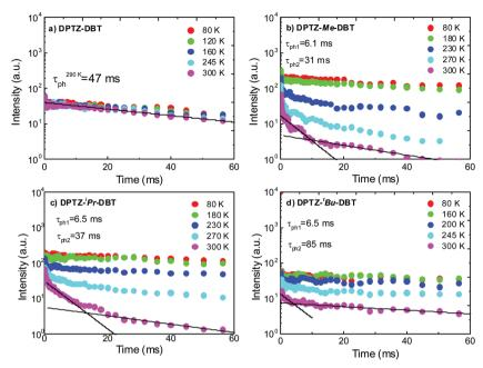
Fig. 8 Time resolved phosphorescence decays in zeonex obtained as a function of temperature for (a) DPTZ-DBT, (b) DPTZ-Me-DBT, (c) DPTZ-iPr-DBT and (d) DPTZ-iBu-DBT.
