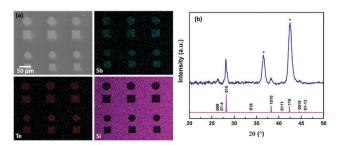
Fig. 1 (a) SEM image with EDX mapping and (b) grazing incidence XRD pattern from Sb<sub>2</sub>Te<sub>3</sub> selectively deposited from [SbCl<sub>3</sub>(Te<sup>n</sup>Bu<sub>2</sub>)<sub>3</sub>] into 30 μm TiN holes and an indexed bulk pattern of Sb<sub>2</sub>Te<sub>3</sub>.42 The TiN substrate peaks are marked by \*.
