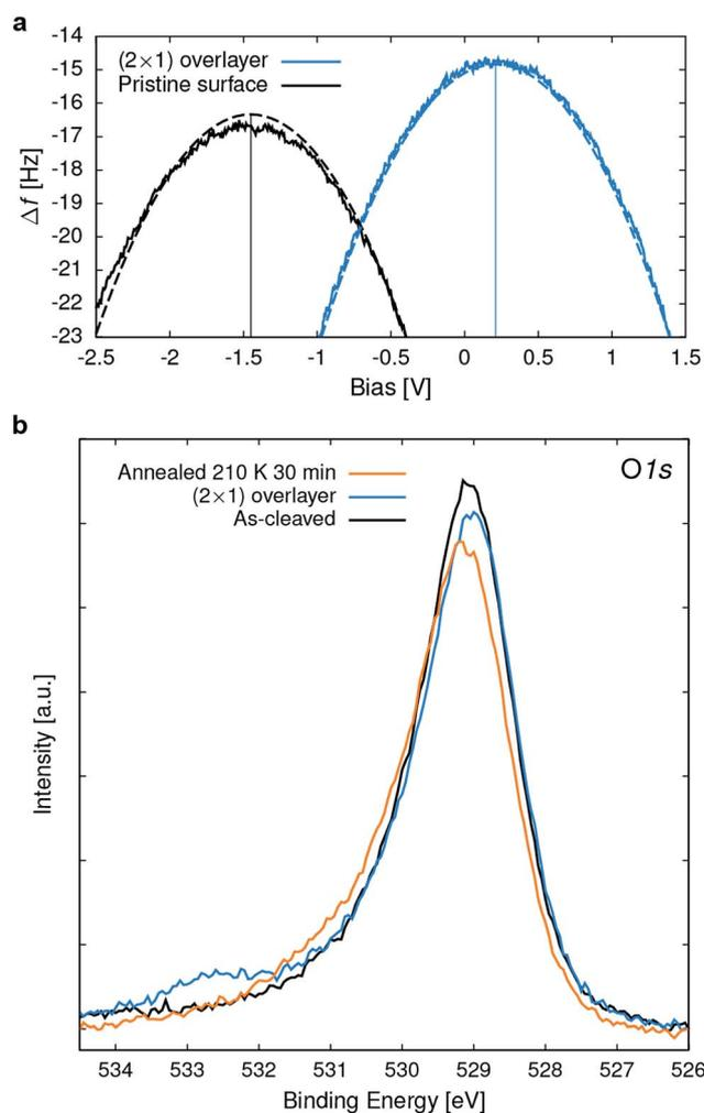
**Fig. 8** Surface spectroscopies. (a) Point Kelvin probe spectroscopy of the pristine surface and the  $(2 \times 1)$   $O_2^-$  overlayer at 78 K. Shown are the measured (full line) and the numerically fitted (dashed lines) Kelvin parabolas, reflecting a change in work function (see main text for analysis details). (b) O 1s XPS (Mg  $K\alpha$ ,  $T_{sample} = 110$  K) spectra of the as-cleaved surface, the  $(2 \times 1)$   $O_2^-$  overlayer and after annealing at 210 K for 30 min.
