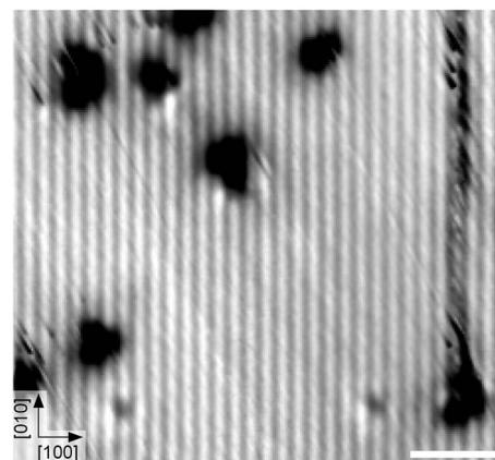
Fig. 4 STM image after dosing 0.025 L O<sub>2</sub> at 110 K. The molecules appear as streaks across point defects. STM parameters: V<sub>sample</sub> = +1.0 V, I<sub>tunnel</sub> = 0.1 nA, T<sub>sample</sub> = 78 K; fast scan direction is 58° clockwise from horizontal. The scale bar corresponds to 3 nm.
