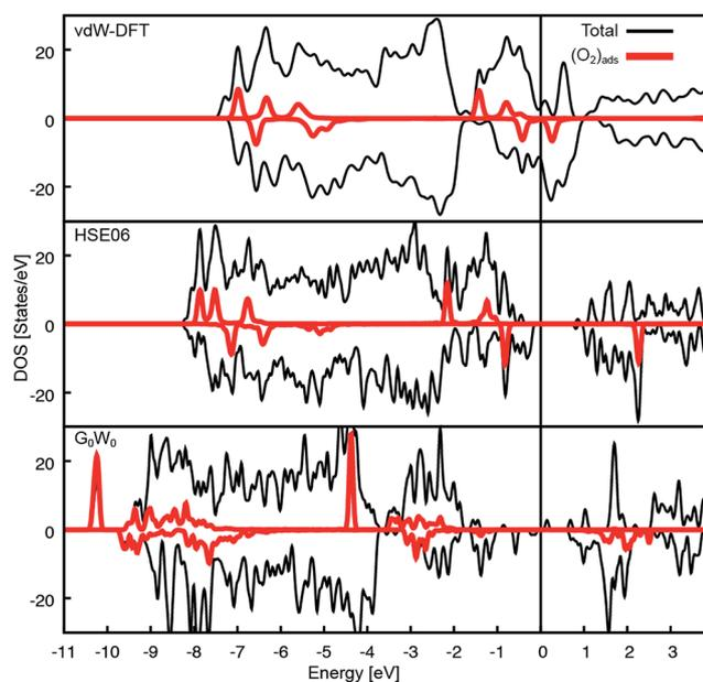
Fig. 6 Density of states for the  $(2 \times 1)$  overlayer. Total and  $O_2$  DOS for the different theoretical approaches. In all cases charge is transferred into the split  $\pi^*$  states of the  $O_2$  in the spin down channel. The HOMO–LUMO gap is 0.7, 3.1 and approximately 1.7 eV on the DFT, HSE06 (insulating phase) and  $G_0W_0$  level, respectively.
