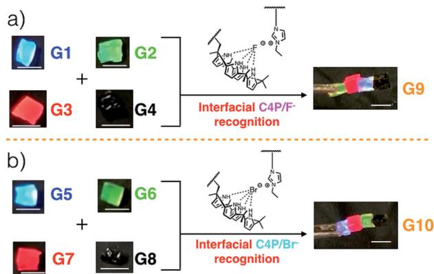
Fig. 1 (a) Multi-fluorescent supramolecular polymeric gel G9 stabilized *via* interfacial C4P/imidazolium-F<sup>-</sup> interactions involving individual blocks of gels G1–G4. (b) Multi-fluorescent supramolecular polymeric gel G10 stabilized *via* interfacial C4P/imidazolium-Br<sup>-</sup> interactions involving individual blocks of gels G5–G8. Scale bar = 0.5 cm.
