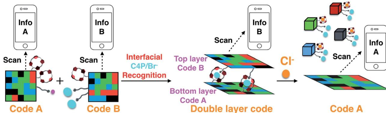
**Scheme 1** Formation of a double layer code construct stabilized *via* presumed interfacial anion-receptor interactions involving the recognition elements present in Code A and Code B. Also shown is the proposed  $Cl^-$  anion induced delamination and encoded information release-based sensing mechanism that allows for chloride specific anion sensing.
