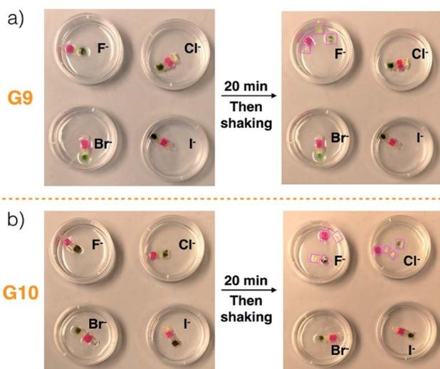
Fig. 3 Photographs of (a) G9 and (b) G10 before and after immersion into chloroform solutions containing various tetrabutylammonium halide anion salts (*viz.* TBAF, TBACl, TBABr, and TBAI) for 20 min. The same concentrations (20 mM) and volumes (20 mL) were used in all cases. The size scale for constructs G9 and G10 is provided in Fig. 1. Disassembled gel blocks are shown using boxes.
