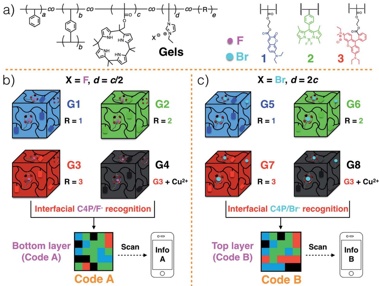
**Scheme 2** (a) Chemical structures of the polymeric gels and the incorporated fluorescent elements. Cartoon representations of: (b) G1–G4 and the formation of 3D colour Code A via interfacial C4P/imidazolium-F<sup>-</sup> interactions; (c) G5–G8 and the formation of 3D colour Code B via interfacial C4P/imidazolium-Br<sup>-</sup> anion interactions.
