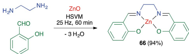
Scheme 46 Mechanochemical synthesis of a zinc-salen complex.
