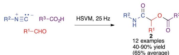
Scheme 2 The mechanochemical Passerini reaction.
