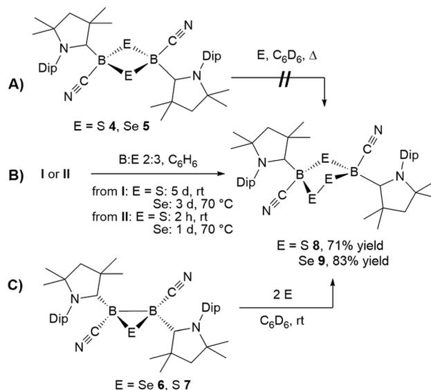
Scheme 7 Unsuccessful ring-expansion of 1,3-dichalcogen-2,4-diboretanes (A) and successful syntheses of 1,2,4-trichalcogena-3,5-diborolanes from **I** or **II** (B) and by ring-expansion of 1,2,3-dichalcogenadiboriranes (C).
