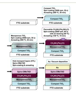
Fig. 1 Schematic illustration of the process used to fabricate the  $CH_3NH_3Pbl_3(Cl)$  photovoltaic cells.
