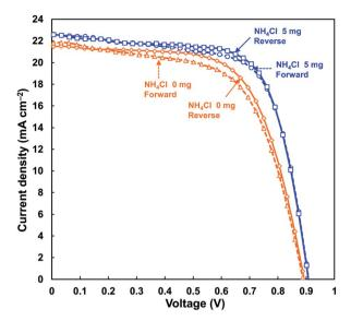
Fig. 2 J-V characteristics of CH<sub>3</sub>NH<sub>3</sub>PbI<sub>3</sub>(Cl) solar cells with and without NH<sub>4</sub>Cl.
