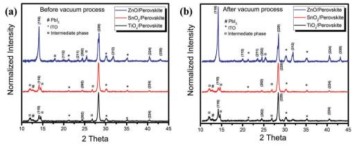
Fig. 2 X-ray diffraction patterns of perovskite films deposited on ZnO, SnO<sub>2</sub> and TiO<sub>x</sub> substrates: (a) before vacuum-processing and (b) after vacuumprocessing. The XRD patterns are all normalized by the (220) peaks located at 28.3°.
