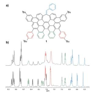
Fig. 2 (a) Structure of 1 and (b) partial  $^1\text{H-NMR}$  spectra (500 MHz,  $C_2D_2Cl_4$ ) of 1 at: 293 K (top) and 369 K (bottom).
