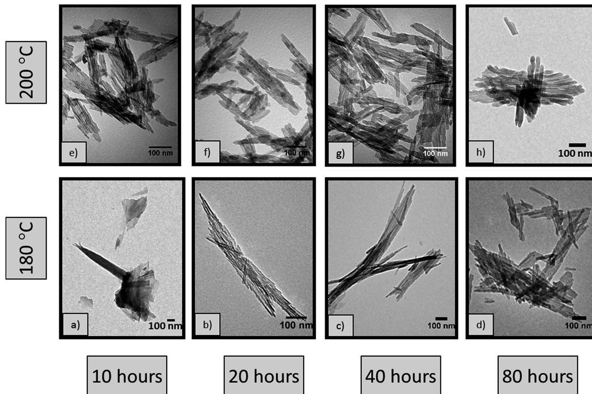
Fig. 6 TEM micrographs of  $\gamma$ - $\text{Al}_2\text{O}_3$  synthesised with 1 M NaOH (0.77 NaOH : Al molar ratio) at 180 °C for (a) 10 hours (b) 20 hours (c) 40 hours (d) 80 hours and at 200 °C for (e) 10 hours (f) 20 hours (g) 40 hours (h) 80 hours.
