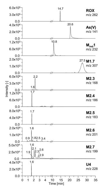
Fig. 3 HILIC separation of electrochemically generated TPs of roxarsone (2200 mV vs. Pd/H<sub>2</sub>). Depicted are the extracted ion chromatograms of all detectable products as well as their retention times ( $t_R$ ).
