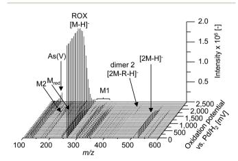
Fig. 1 Mass voltammogram (m/z 100-600) of roxarsone obtained with ESI(-)-MS in the potential range 0-2500 mV vs. Pd/H<sub>2</sub>. R = +20+ NH - 4H - HAsO<sub>3</sub>.
