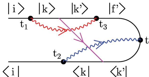
Fig. 3 An example of an optical scattering process in junction.  $|i\rangle$  and  $|k\rangle$  are eigenstates of a neutral molecule, and  $|k'\rangle$  and  $|f'\rangle$  are eigenstates of a cation. Wavy lines (red and blue) represent photon Green functions (11), and the straight line (magenta) indicates electron self-energy due to coupling to contacts (12).
