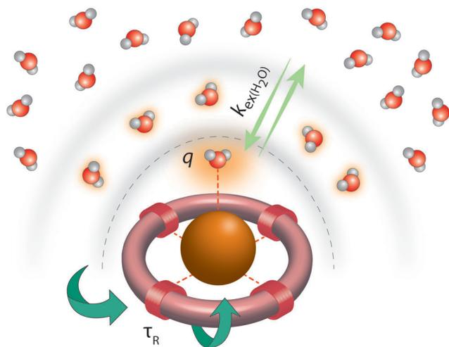
Fig. 3 In activatable,  $T_1$ -weighted MRI contrast agents, MR signal change can be generated *via* modulation of the main parameters that determine relaxivity: the number of water molecules directly coordinated to the paramagnetic ion ( $\text{Gd}^{3+}$ ),  $q$ ; the exchange rate of the inner sphere water with bulk water,  $k_{\text{ex}(\text{H}_2\text{O})}$ ; the rotational motion of the complex, characterized by the rotational correlation time,  $\tau_R$ .
