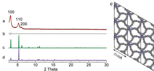
Fig. 2 (a) Experimental (black) and refined (red) PXRD patterns of **HAT-NTBCA-COF**, (b) difference plot between the experimental and refined PXRD patterns, and simulated PXRD patterns of the COF with (c) AA and (d) AB stacking, and (e) the unit cell structure of **HAT-NTBCA-COF** in AA stacking.
