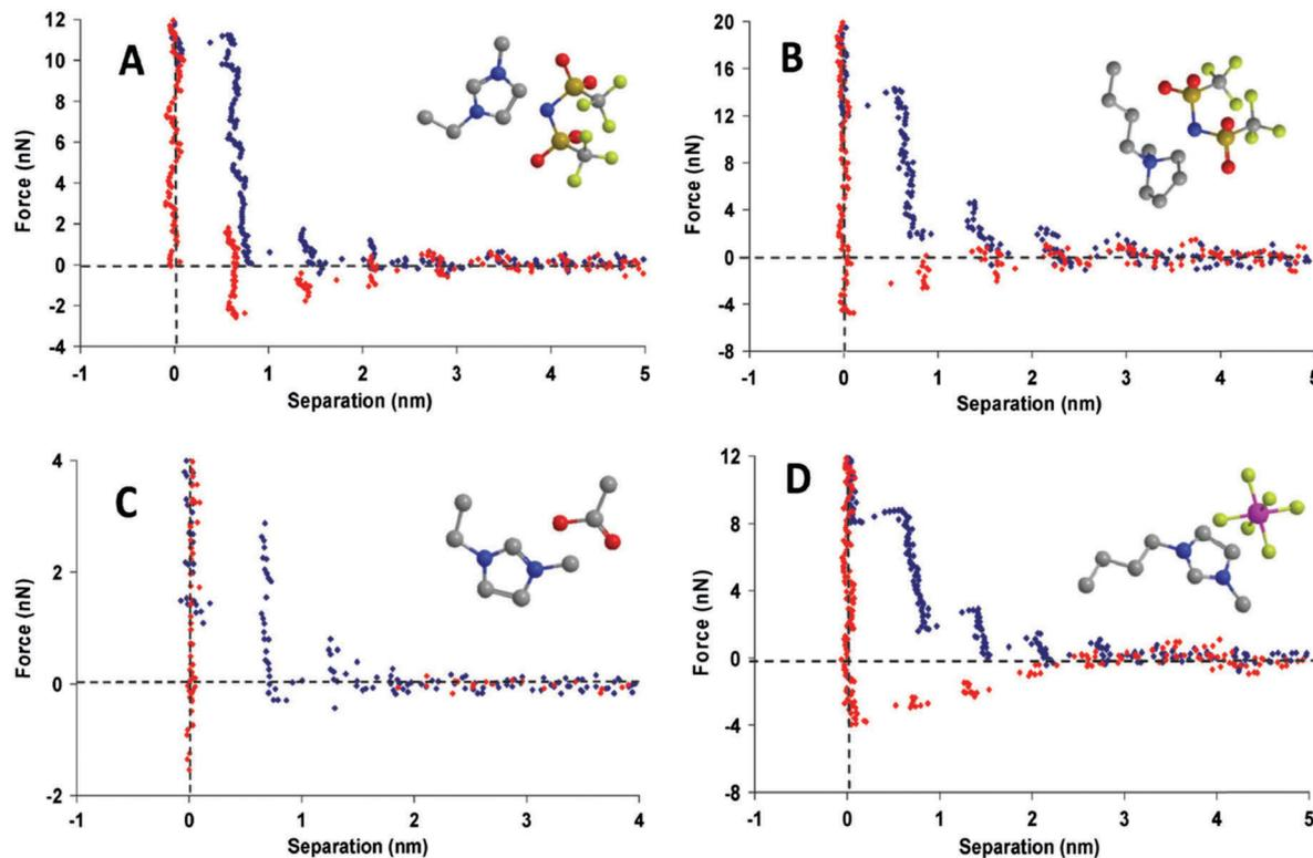
Fig. 3 Force-distance profile for a  $\text{Si}_3\text{N}_4$  AFM tip approaching (blue) and retracting from (red) a mica surface in (A)  $[\text{C}_2\text{mim}^+][\text{NTf}_2^-]$ , (B)  $[\text{C}_4\text{mpyr}^+][\text{NTf}_2^-]$ , (C)  $[\text{C}_2\text{mim}^+][\text{NTf}_2^-]$ , and (D)  $[\text{C}_4\text{mim}^+][\text{PF}_6^-]$ . Reproduced from ref. 24 with permission from the PCCP Owner Societies.
