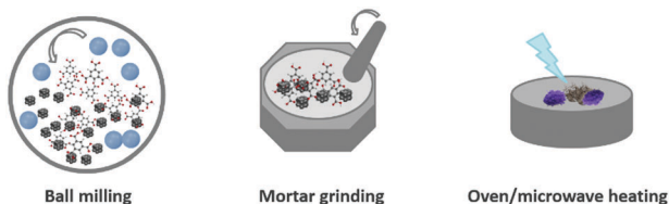
Fig. 3 Schematic diagrams illustrating the solvent-free synthesis of MOFs from solid matters.
