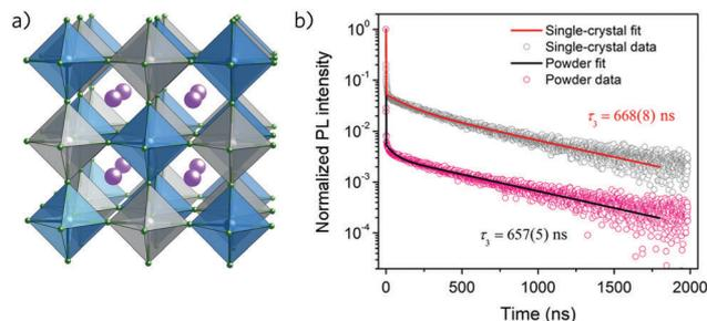
**Fig. 9** (a) Crystal structure of  $\text{Cs}_2\text{BiAgBr}_6$ . Adapted with permission from ref. 427. Copyright 2015, American Chemical Society. (b) Time-resolved room temperature photoluminescence (PL) of single-crystal and powder  $\text{Cs}_2\text{BiAgBr}_6$ , including fits for the PL decay time ( $\tau$ ). Reprinted with permission from ref. 428. Copyright 2016, American Chemical Society.
