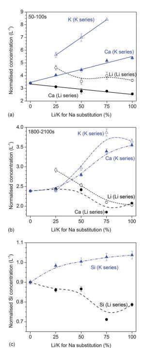
Fig. 6 Dynamic dissolution: normalised concentrations of modifier ions at (a) the initial peak (50 to 100 s) and (b) the final stage of the experiment (1800 to 2100 s). (c) Normalised concentrations of silicon ions at the final stage of the experiment (1800 to 2100 s). Solid lines are linear regression; Li series:  $R^2 = 0.926$  (Ca); K series:  $R^2 = 0.980$  (Ca), 0.999 (K).
