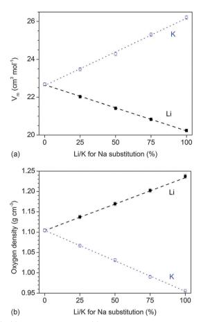
Fig. 8 (a) Molar volume,  $V_{\rm m}$ , and (b) oxygen density, a parameter describing the compactness of the silicate network, vs. Li/K for Na substitution in the glass. Lines are linear regression:  $R^2(V_m) = 0.999$  (Li), 0.998 (K);  $R^2$ (oxygen density) = 0.999 (both Li and K)
