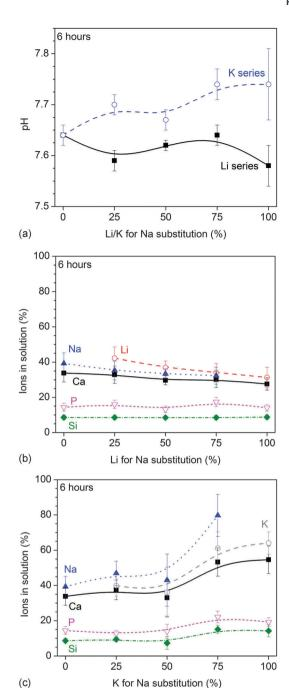
Fig. 1 Static dissolution experiments: (a) pH and (b and c) relative ionic concentrations vs. (b) Li and (c) K for Na substitution at 6 hours of immersion in Tris buffer.
