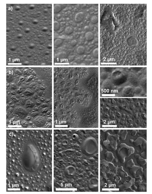
Fig. 7 SEM micrographs of glass samples (a) Li25, (b) Li100, and (c) K100 left in ambient atmosphere for 0 days (left), 2 days (centre) and 7 days (right).
