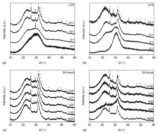
Fig. 4 XRD patterns of glasses (a) Li75 and (b) K75 at various time points of immersion in Tris buffer and (c) Li and (d) K for Na substituted glasses at 24 hours of immersion in Tris buffer (\* apatite, \* calcium carbonate; static dissolution experiments)
